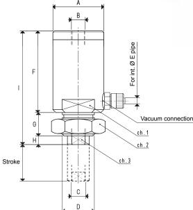
The cylinders described in this page are vacuum operated. By creating vacuum in the cylinder front chamber, the stem, which is solidly connected to the piston, comes out overcoming the opposing spring force.
